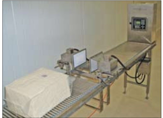
MoistScan MA600 measures moisture in cheddar blocks for quality control purposes at an Australasian plant.
